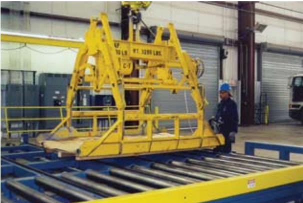
Most systems accumulate 3 to 4 finished skids for efficient pick up by crane or fork truck. Crane time and travel time is reduced by moving 3 or 4 skids at a time to the shipping dock. Productivity increases of 15 to 30 percent have been obtained in systems installed by Canrack
