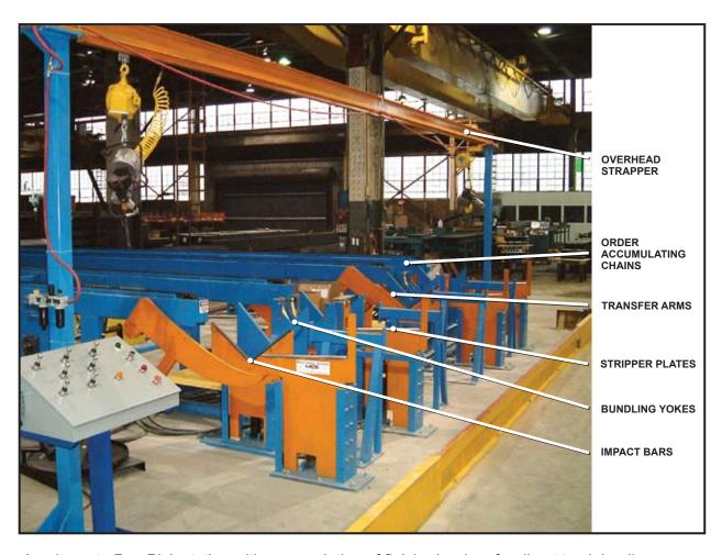
An alternate Pan Pick station with accumulation of finished orders for direct truck loading or transfer to laydown. This provides immediate clearing of the station when an order is finished and is not dependant on crane or fork truck to begin packaging the next order.
