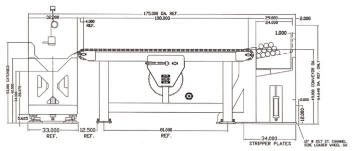
Typical Pan Pick station with accumulation of material for orders feeding impact bars, bundling yokes and packaging station. This provides a buffer between sideloader and packaging increasing productivity
