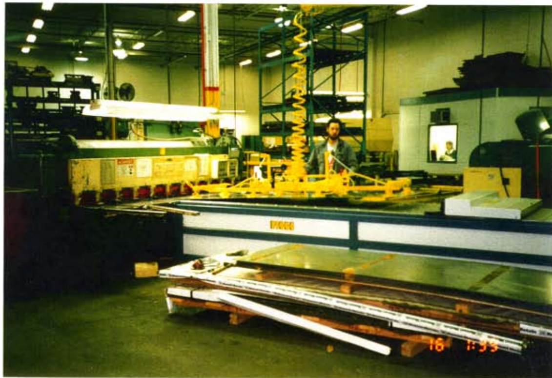
SHEET IS QUICKLY AND GENTLY LOWERED INTO JAWS OF CNC SHEAR FEEDER
