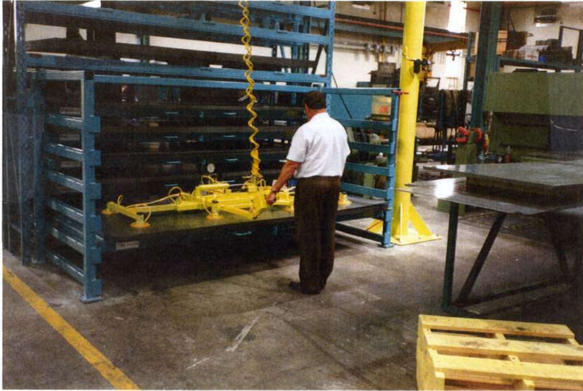
SHEETS ARE PICKED FROM A 6 DRAWER STORAGE RACK (EACH DRAWER CAPABLE OF HOLDING 5,000 LBS. OF SHEETS)
