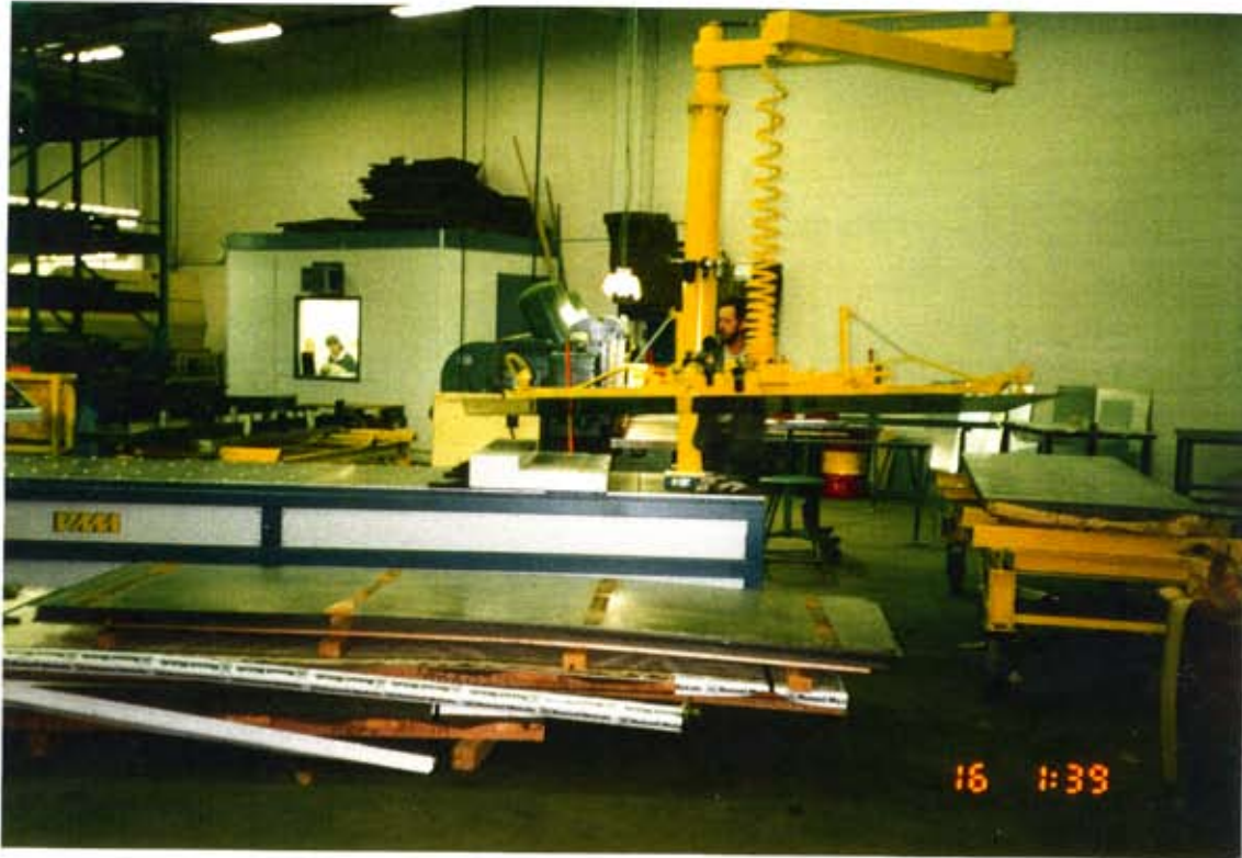
ONE MAN LIFTS 600 LB. SHEET WITH CANRACK SHEET HANDLER
