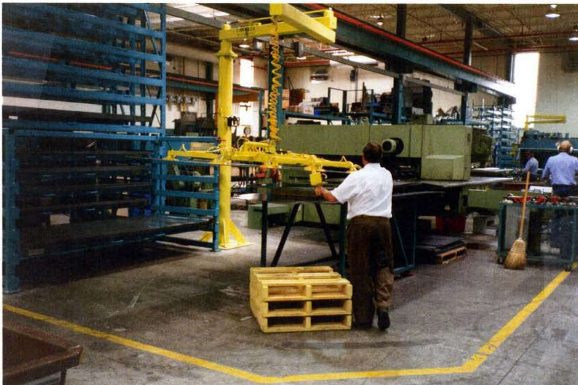
SHEETS ARE EASILY MOVED TO THE C.N.C. MACHINE AND PLACED INTO THE MACHINE GRIPPERS
