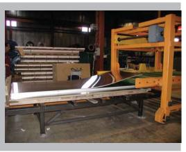
The Bundle Splitter® moves away from the customer skid and packaging can be completed on the pack table. Optional conveyors may be added to allow one person to operate the Bundle Splitter® and a second operator to package which will allow the sideloaders/fork trucks to continually run a finished package can be achieved every 3 minutes when using 2 operators.
