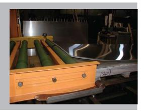
The sheets are transferred to the Bundle Splitter® scratch free and hands off with the operator using a hand held remote control. Material loads onto the Bundle Splitter® on covered power driven rollers.
