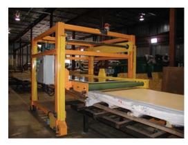
The Bundle Splitter® moves over the customer skid and places the material on the skid. All functions are controlled with a hand held remote and the material is correctly aligned with the customer skid. The complete cycle takes 2 minutes or less.
