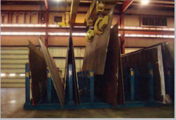
The magnets are released from the plate with a discharge switch on the remote control. A fanning switch on the control also controls the depth of magnetic field to allow picking one plate at a time.
