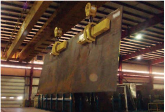
Plates are lowered into the racks while the operator is standing clear. The racks use a specially designed base plate to force the plates close stacked to the other plates in the pocket.
