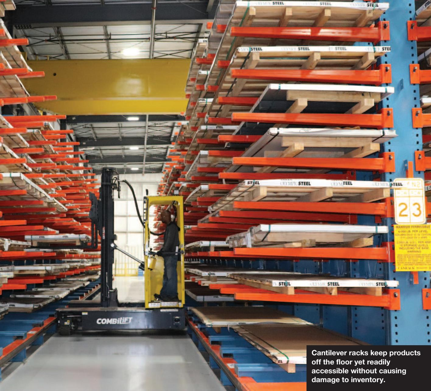
**Cantilever racks keep products off the floor yet readily accessible without causing damage to inventory.**
