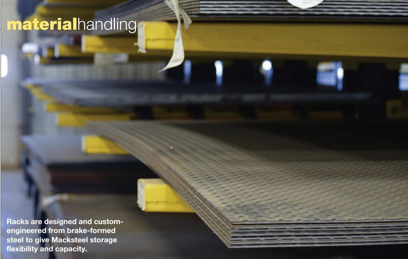
Racks are designed and custom-engineered from brake-formed steel to give Macksteel storage flexibility and capacity.
