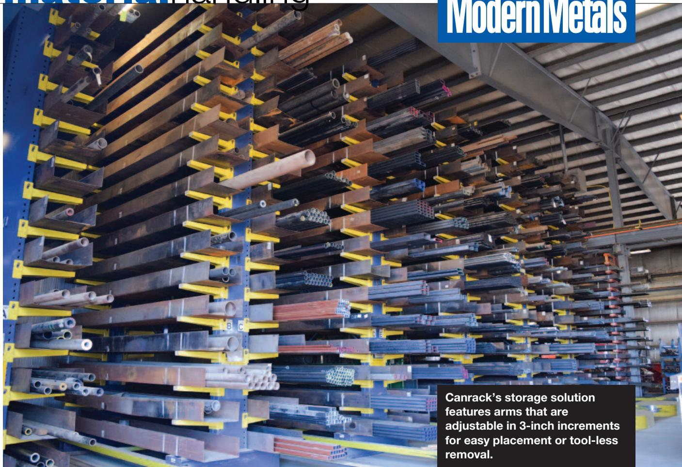
Canrack's storage solution features arms that are adjustable in 3-inch increments for easy placement or tool-less removal.
