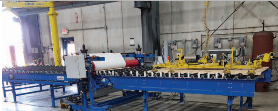
The line can handle high-tack films and has built-in lift equipment for safer operation and increased productivity.
