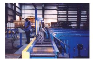
Bundling straps cinch the material into a tight bundle for strapping. The operator has hydraulic controls allowing him to rotate and compress the material to achieve nesting of material and make square bundles for squares, rectangles and flats.
