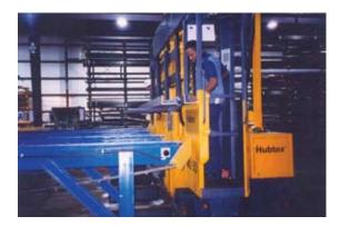
Picked orders are brought to the station on the forks of a sideloader and placed on the accumulating chain conveyor. Separation wedges allow several orders to be placed with separation between each order. This can allow banding of individual lines which can then be banded into the complete order.
