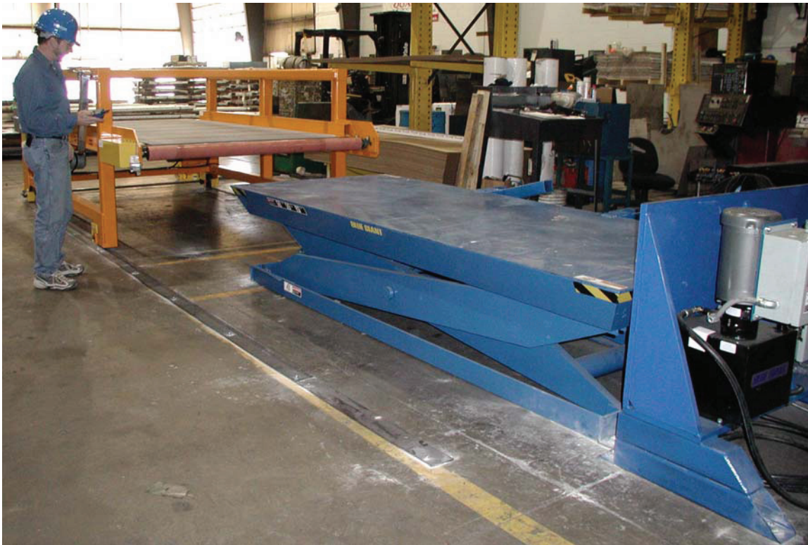
Sheet Order Filling Low Volume Bundle Splitter® - BS660LV installed at customer facility in Indianapolis.
