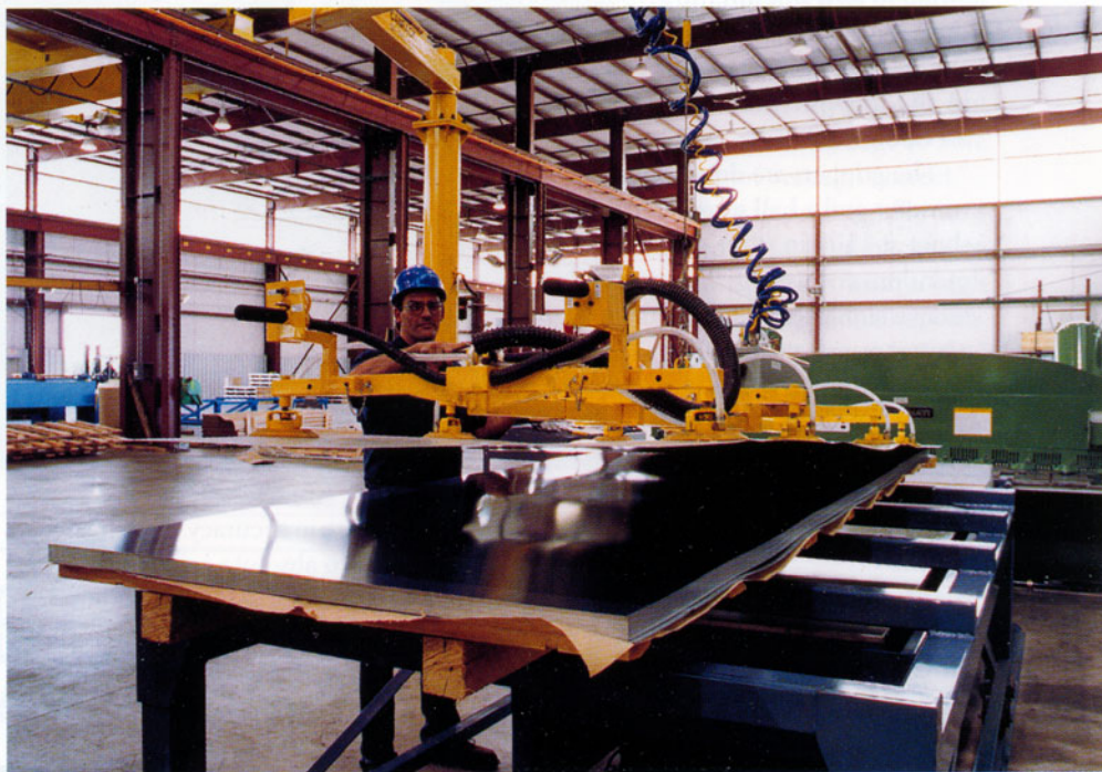
Carey Dye transfers a sheet to Ryerson Tull's automated shear feeder with a Canrack vacuum sheet handler. The double-articulated handler has a sensing device that will not allow the load to be released as long as there is tension on the lift cable. Photographs by the author.
