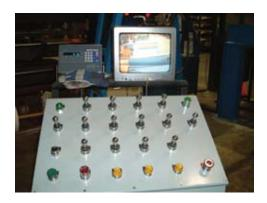
A control panel and the use of hydraulic soft start valves gives the operator perfect control on all machine movement. Manual or automatic modes give flexibility and in automatic mode relieves the operator to quickly begin processing the next order. Video screens mounted on the panel assists the operator with vision control of all elements where additional visibilty is required.
