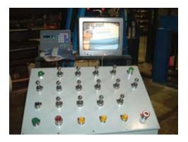
A control panel and the use of hydraulic soft start valves gives the operator perfect control on all machine movement. Manual or automatic modes give flexibility and in automatic mode relieves the operator to quickly begin processing the next order. Video screens mounted on the panel assists the operator with vision control of all elements where additional visibility is required.
