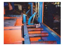
Bundling straps rotate and manipulate the material into a tight bundle for strapping. The operator uses hydraulic controls for movement and rarely has to touch the material with his hands. Shapes can be nested and compressed and squares, rectangles and flats can be formed into square bundles.
