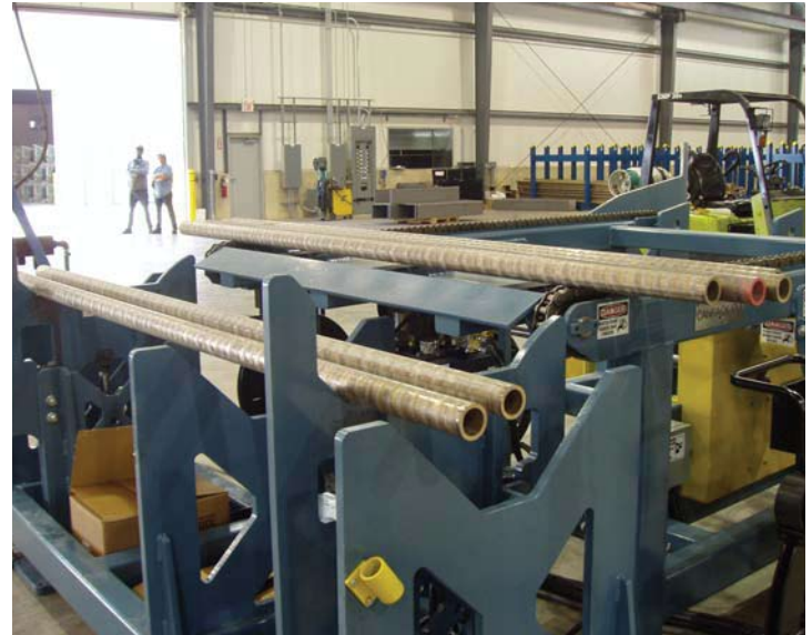
Banding station with impact bars and bundling yokes
