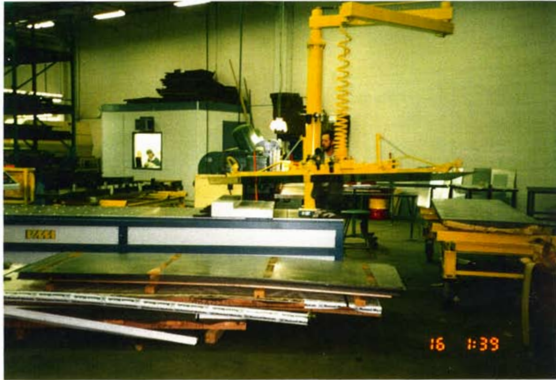
ONE MAN LIFTS 600 LB. SHEET WITH CANRACK SHEET HANDLER
