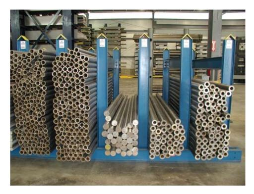
Structural steel stanchion racks offer an economical solution to store bulk reserve stock or storage for high volume items that can be order selected by crane. The racks are manufactured in 20' modules and shipped knocked down for efficient shipping costs. The different sections bolt together on site without the need for any welding or special tools.
