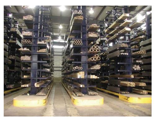
Welded fixed arm structural steel Cantilever Racks are available to 40' tall with arms from 24" to 72" long. The selection of most economical structural sections based on applicable design criteria can make structural racks the least cost per load stored.
