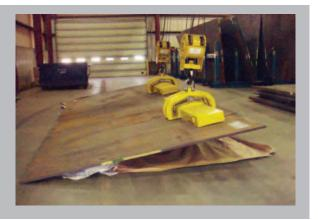
Plates are securely held by the magnets with control from the operator using his crane remote control. At no time is the operator near the plate or racks for improved operator safety.
