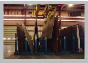
The magnets are released from the plate with a discharge switch on the remote control. A fanning switch on the control also controls the depth of magnetic field to allow picking one plate at a time.
