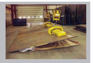
Plates are securely held by the magnets with control from the operator using his crane remote control. At no time is the operator near the plate or racks for improved operator safety.
