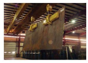
Plates are lowered into the racks while the operator is standing clear. The racks use a specially designed base plate to force the plates close stacked to the other plates in the pocket.
