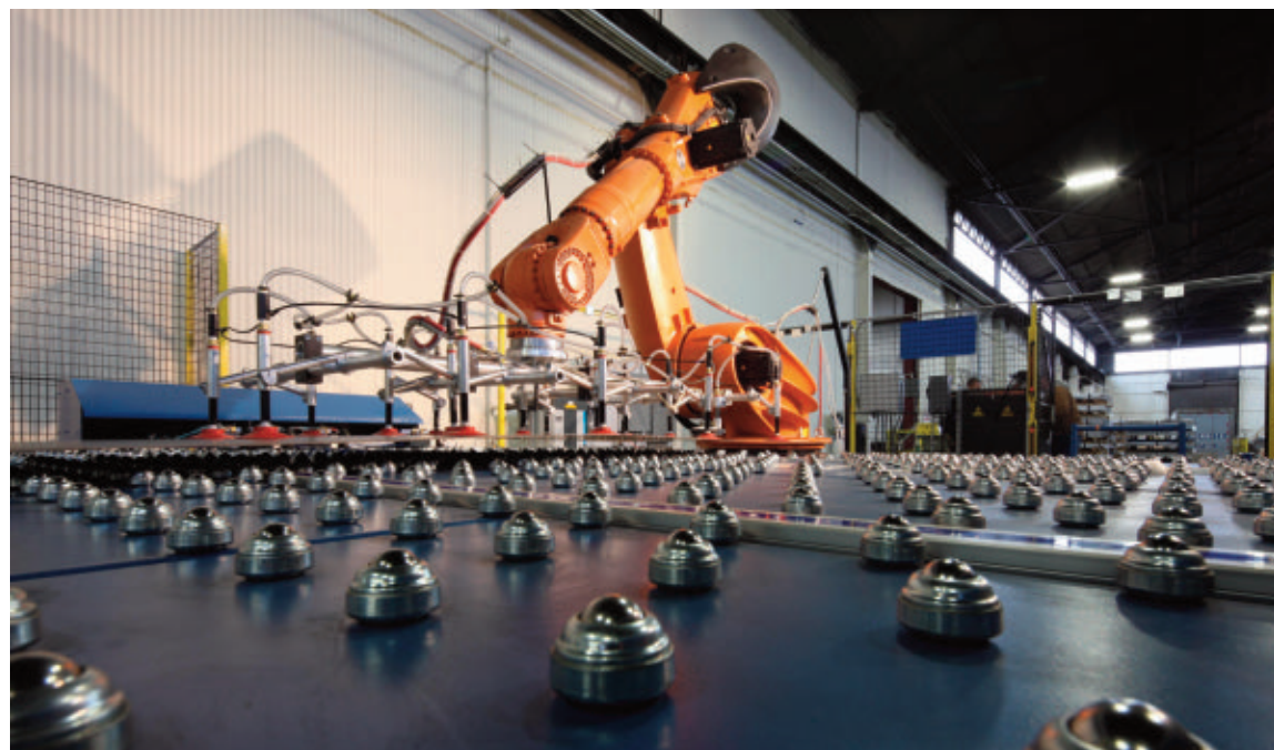
FIGURE 3 Four servo-driven clamps at the raised blue housing, shown here immediately behind the sheet being placed onto the table, position the blank for shearing within \pm 0.005 in.
