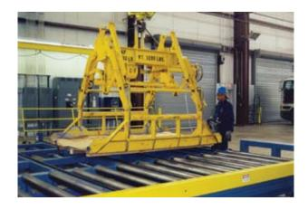
Most systems accumulate 3 to 4 finished skids for effecient pick up by crane or fork truck. Crane time and travel time is reduced by moving 3 or 4 skids at a time to the shipping dock. Productivity increases of 15 to 30 percent have been obtained in systems installed by Canrack
