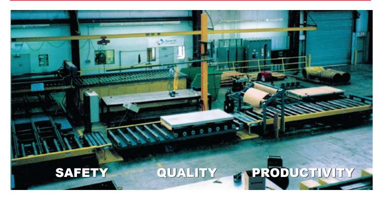
CTL productivity increases can be realized by increasing run time through efficient skid entry and removal from the stacker. Most CTL systems require packaging on line or removing skids and transporting them to a packaging station. This often leads to an accumulation of pallets to be banded and loss of efficient production.
