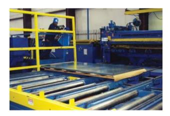
Pallets exit with CTL stacker and transfer to the interface unit of the packaging system. The pallet movement is now under computer control which accumulates several pallets to feed the banding station
