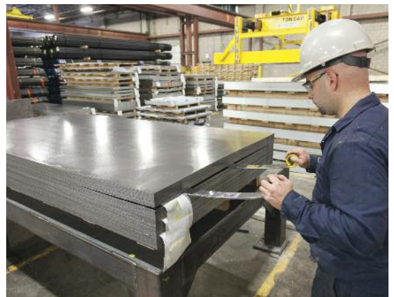
The operator inserts Canrack’s pick and split wedges to indicate where to separate the stack of sheet metal.
